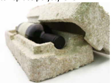
Mushroom-based packaging material from www.ecovatedesign.com that could help replace plastic foam products.
